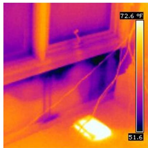
Infrared Image Water Leak below Window
